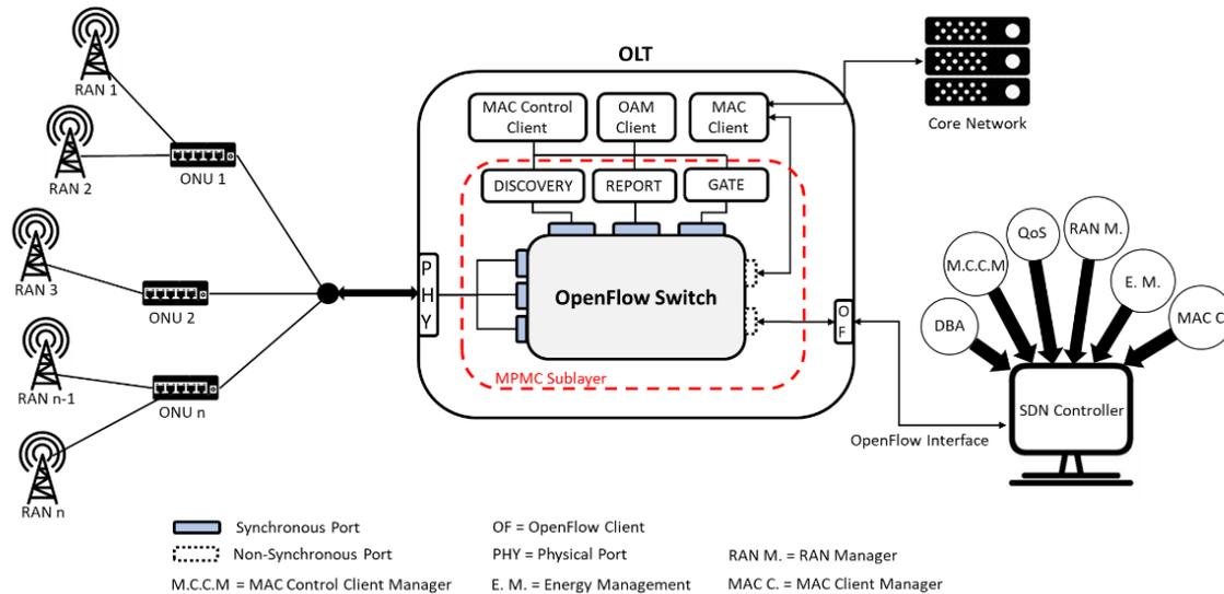
Figure 1. SDN-based 5G EPON Architecture.
